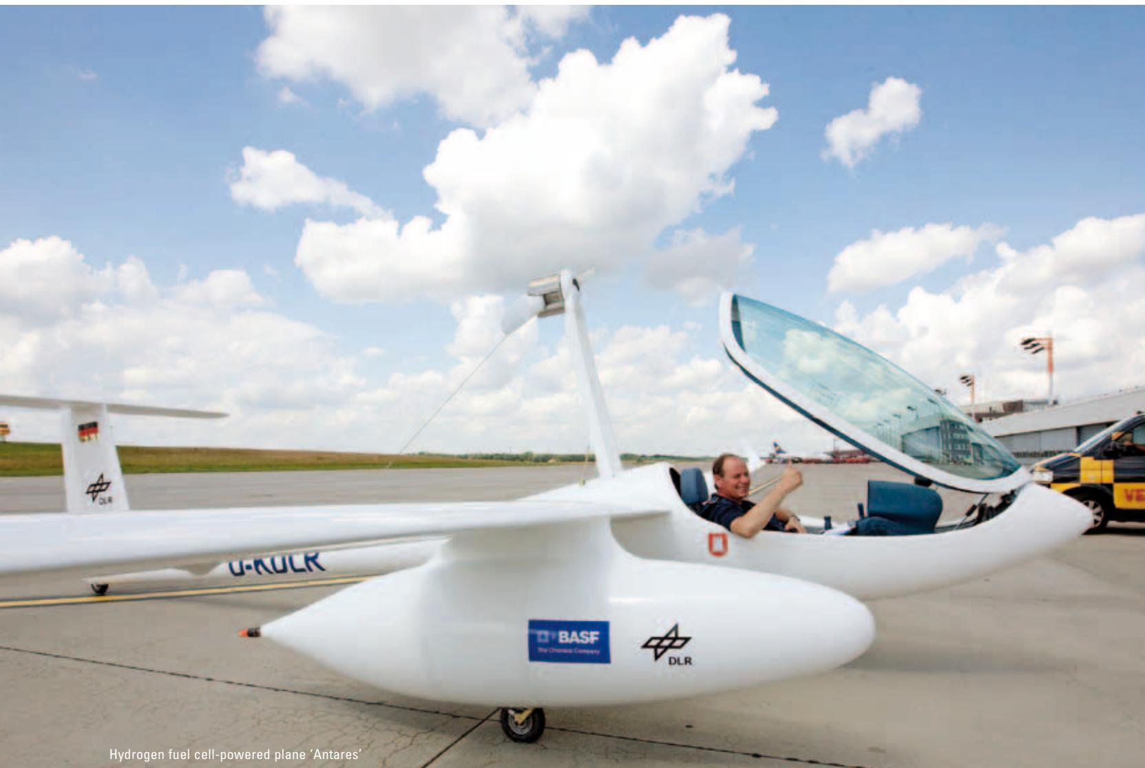
Hydrogen fuel cell-powered plane 'Antares'
